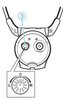
The balance control allows for right/left balance adjustment. Adjust the balance so that you can hear equally well with both ears.
